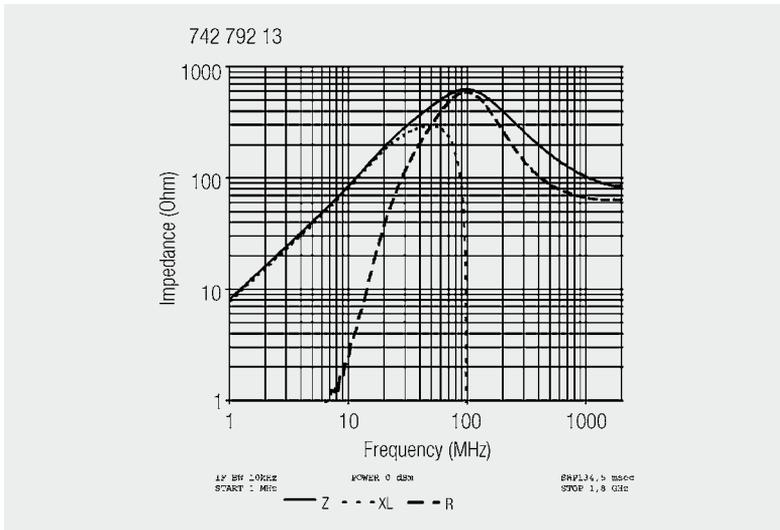
Fig. 2.5: Impedance curve for the SMD ferrite 742 792 13
